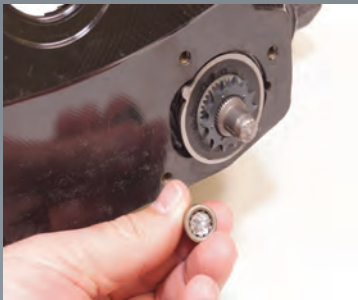
Failed adjuster / Requires caliper replacement
